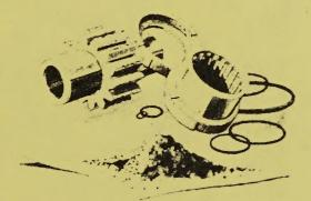
The best thing to do after you have replaced a failed component is to clean the system thoroughly before you put it back on the job.
